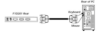
**4.** Connect the female end of the VGA cable to the male VGA input port on the back of the Reverse KVM Switch.
